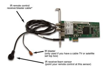
The IR remote control receiver/blaster cable has two ends: the IR receiver/learn sensor and the IR blaster:
