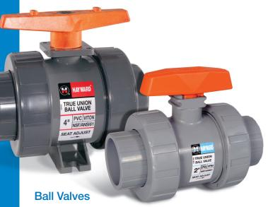
Full range of thermoplastic ball valves in PVC, CPVC and GFPP materials from sizes 1/2" – 6". Features True-Union design with socket, threaded or flanged end connectors. Also includes 3-way Horizontal and Lateral ball valves in PVC and CPVC. All valves designed for easy actuation. Pressure rating of 250psi/150psi at 70°F non-shockup through 2" and 235psi/150psi at 70°F non-shock up through 4".
