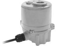
**HZSN Series:** Compact, reversing, non-spring return actuator is ideal for limited space applications and smaller size ball valves. Standard 24VAC/VDC and 85-265VAC supply, manual override including lock-out function (lever operated), and open/ close or proportional control. Lightweight, aluminum alloy electrostatic coated, NEMA 4X and Class B motor protection. LED Pwr/Open/Close indicators & 1 M wiring cable standard.
