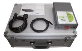
Together with the included ATS adjusting and testing software, the PWM 20 phase angle measuring unit serves for diagnosis and adjustment of HEIDENHAIN encoders. The PWM 20 is the successor of the IK 215 and consists of the following components:
