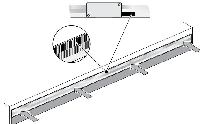
Starting from the middle, press the scale tape evenly onto the mounting surface using a roller.
