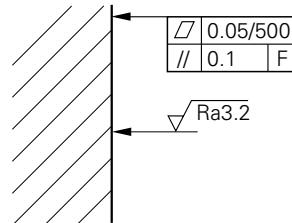
The mounting surface must be free of paint, dust, or grease.
