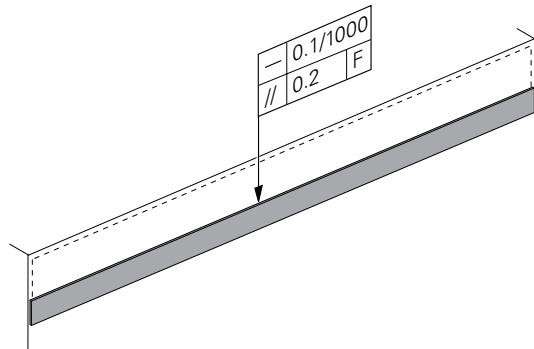
The scale tape with the PRECIMET adhesive mounting film has to be attached at a temperature  $> 15^{\circ}\text{C}$ ! Pay attention to the expiration date on the package! Peel off the protective film from the mounting film, protect the adhesive surface from contamination!
