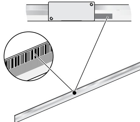
Insert the scale tape in the scale-tape carrier (do not bend it), then secure the scale tape with fixing clamp.
