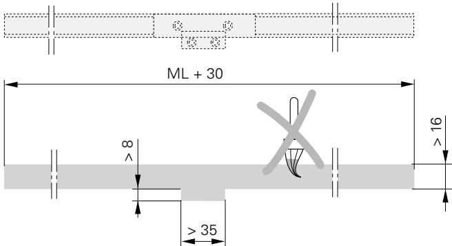
The scale tape carrier with PRECIMET adhesive mounting film has to be attached at a temperature  $> 15^{\circ}\text{C}$ ! Pay attention to the expiration date on the package! Peel off the protective film from the mounting film, protect the adhesive surface from contamination!
