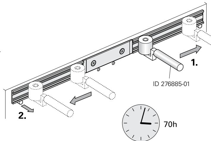
Ensure that the position of the absolute track is correct: Absolute track is above incremental track if cable outlet is at right.
