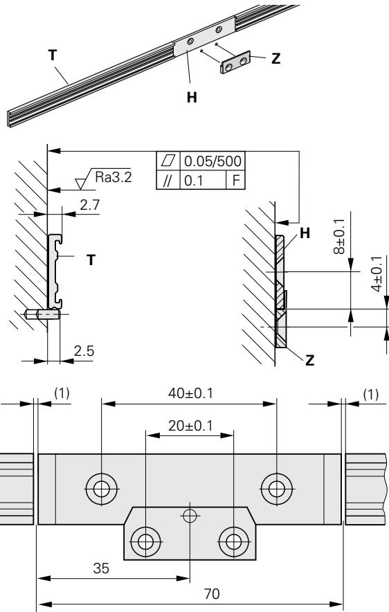
Attach the stop pins or the stop rail.
