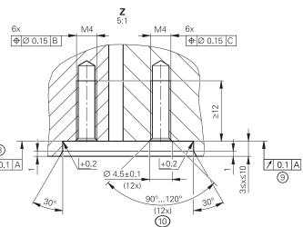
Tolerancing ISO 8015 ISO 2768 - m H < 6 mm: ±0.2 mm
