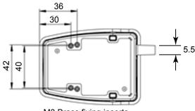
M3 Brass fixing inserts Bottom holes as standard
