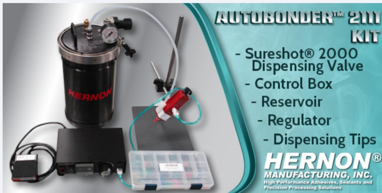
Take your manufacturing to the next level with customized dispensing systems. *HERNON®* specializes in solving problems with a unique Total Solutions approach. By manufacturing both the adhesive materials in this catalog and building custom dispensing solutions, *HERNON's* expert engineers can retrofit specialized manufacturing solutions into your assembly line with a precision that can't be matched by companies that only make a part of the solution.
