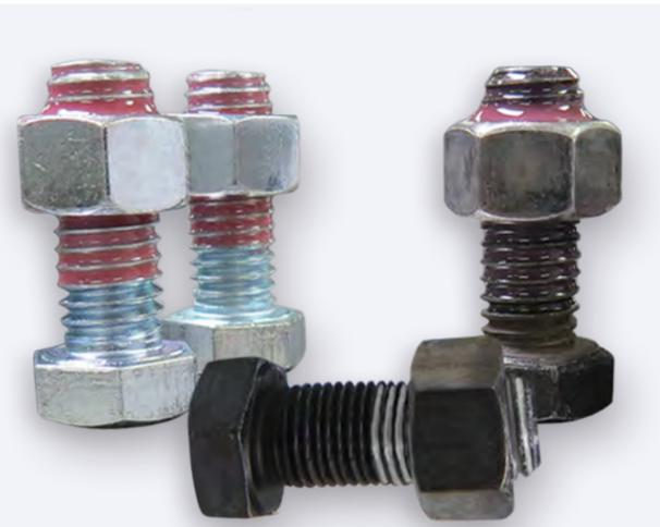
HERNON® offers a complete line of **Nuts N' Bolts®** adhesives & sealants. These anaerobic adhesives are designed for use with assemblies with threaded fasteners. They are single component, 100% active liquids that self-harden when air is omitted such as between the mating surfaces of a nut and bolt, while remaining a stable liquid in its container.
