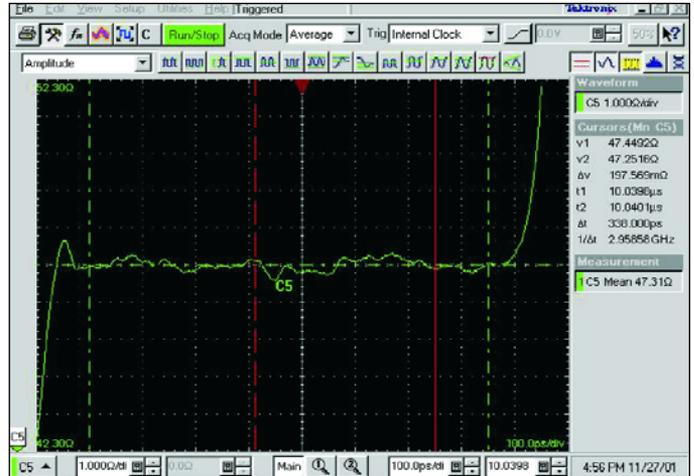
Figure 10 · This measurement window has a narrower scale than Figure 9, showing TDR measurement results for the length of transmission line between the two discontinuities.
