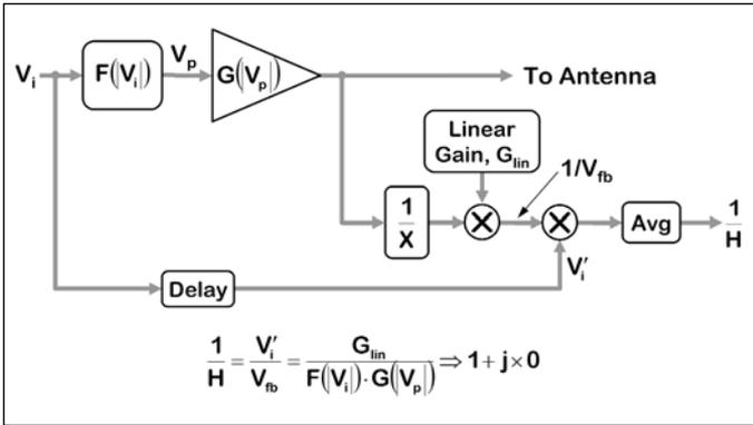
Figure 5 · Implementation of the adaptation algorithm.
