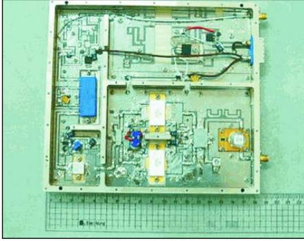
**Figure 11** . The 30 W<sub>rms</sub> power amplifier developed for the linearization experiments.
