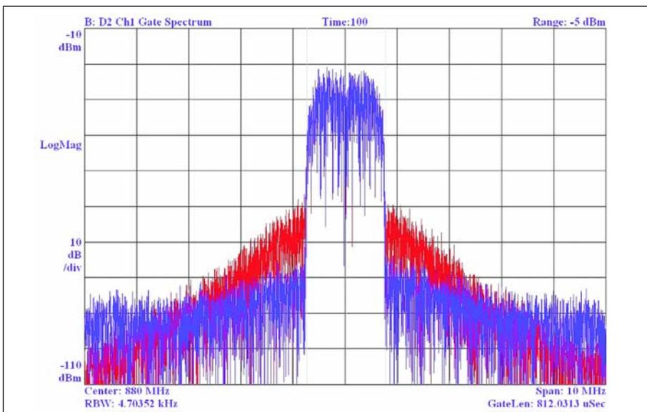
**Figure 12** . PA output with and without DP of the actual hardware PA (Red: without predistortion, Blue: with predistortion).
