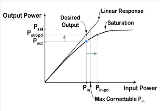
Figure 2 · Power amplifier  $P_{out}$  versus  $P_{in}$  and digital predistortion.
