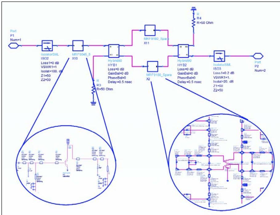
Figure 7 · The PA block diagram defined in ADS.
