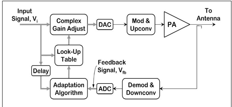
Figure 3 · Digital predistortion block diagram.
