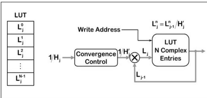
Figure 6 · Calculation of new predistortion function.
