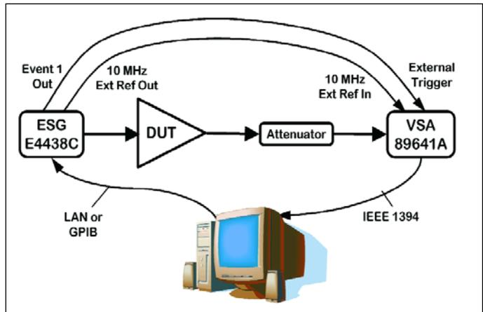
Figure 10 . ESG, VSA, and PC hardware set-up in the connected solution.
