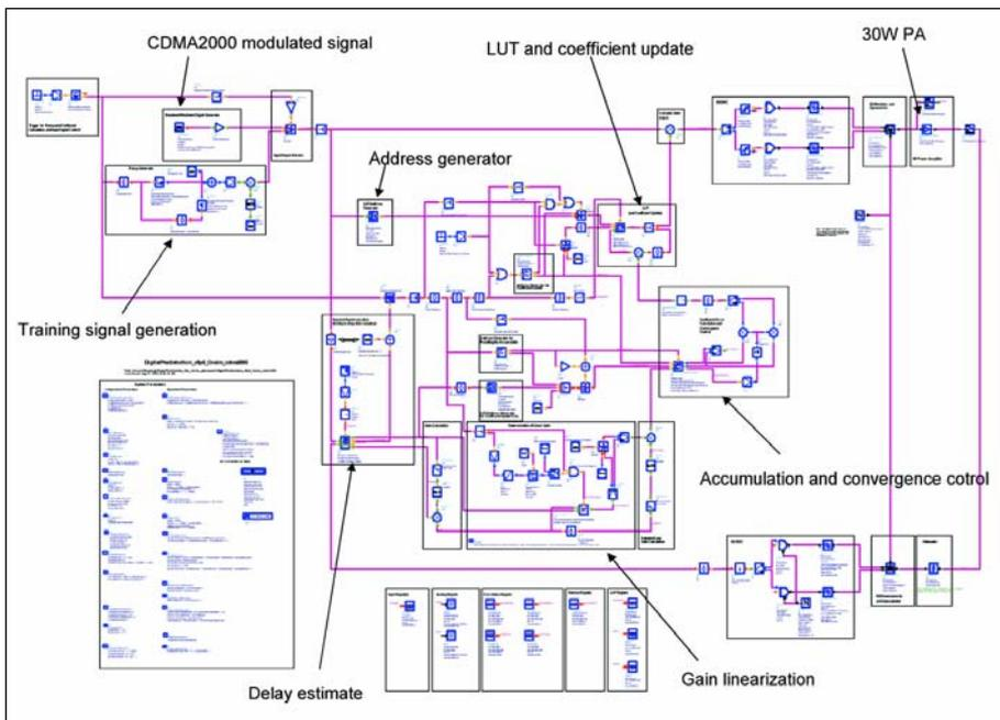
Figure 8 · The complete simulation schematic of the digital predistortion linearizer.
