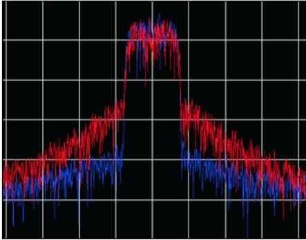
**Figure 9** - PA output with and without DP of the modeled PA in ADS (Red: without predistortion; Blue: with predistortion).
