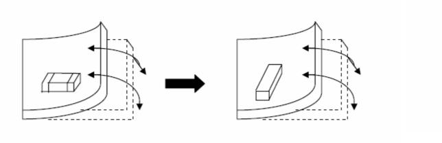
(2) Component layout close to board separation point. Susceptibility to stress in the order: A > C > B = D
