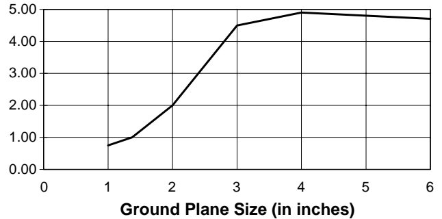
Figure 4: Antenna Zenith Gain vs. Ground Plane Size
