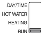
A green **INDICATOR LAMP** shows when the heating or hot water is switched **ON**.
