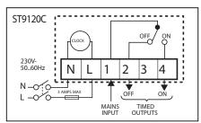
Just replace existing timeswitch, fits directly on to many other timeswitch backplates. No power supply required to thermostat.
