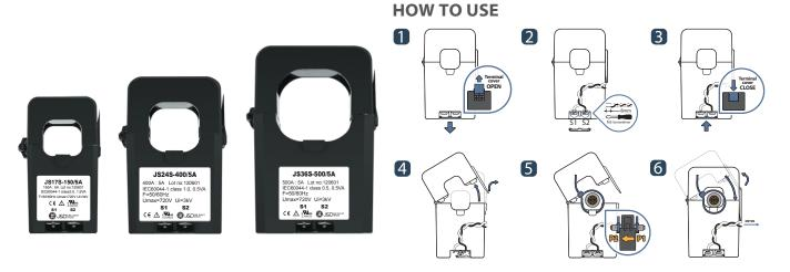
JS series of split-core current transformer offers 5A at secondary from sensed primary current for metering application. It can be used for power meter, distribution system, control panels, switchgear and other equipment. It is designed to install to live power line without disconnection as split-core compact type. Also, over-voltage protection circuit is included to offer safe, fast and cost effective installation.
