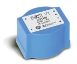
JIVD50 is designed for direct measuring as PCB mounted type. These VTs offer an optional transformation between input and output voltage. Input is available from 300V - 600V and output is from 100mV - 7V by customer needs. These VTs are the best solution for high accurate measuring of voltage.
