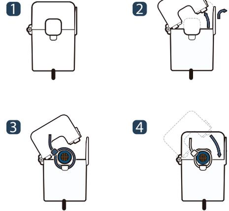
JS series of split-core current transformer offers 333mV at secondary from sensed primary current. Without using secondary CT inside of meter, users directly connect JS series to a meter for high accuracy metering application. It enables one meter to be adopted for various current rating by only changing primary CT so it makes compact design meter and reduces developing cost. Also, over-voltage protection circuit is included to offer safe, fast and cost effective installation.
