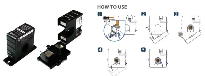
JM21N series of split-core current transformer offers 1A at secondary from sensed primary current. Without using secondary CT inside of meter, users directly connect JM21N series to a meter for high accuracy metering application. It enables one meter to be adopted for various current rating by only changing primary CT so it makes compact design meter and reduces developing cost. Also, over-voltage protection circuit is included to offer safe, fast and cost effective installation.
