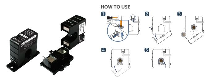
JM21X series of split-core current transformer offers 333mV at secondary from sensed primary current. Without using secondary CT inside of meter, users directly connect JM21X series to a meter for high accuracy metering application. It enables one meter to be adopted for various current rating by only changing primary CT so it makes compact design meter and reduces developing cost. Also, over-voltage protection circuit is included to offer safe, fast and cost effective installation.
