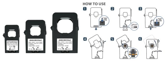
JS series of split-core current transformer offers 333mV at secondary from sensed primary current. Without using secondary CT inside of meter, users directly connect JS series to a meter for high accuracy metering application. It enables one meter to be adopted for various current rating by only changing primary CT so it makes compact design meter and reduces developing cost. Also, over-voltage protection circuit is included to offer safe, fast and cost effective installation.
