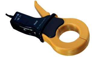
Clamp and compact, the AC/DC current probe model JCP52 is the ideal complement for any multimeter to measure AC/DC current in low-power with secondary, 0-5V 0-10V DC output. With its two ranges, it offers excellent resolution for measuring AC intensities from 1mA to 1000A and DC intensities from 100mA to 1200A.
