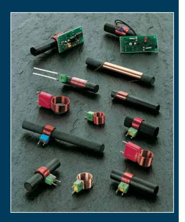
High-grade industrial modules receive data from the PTB (Physikalische Technische Bundesanstalt = German Federal Institute for Physical Technology) in Mainflingen. The antennas are manufactured from high quality ferrite cores and capacitors. Using the latest measurement technology, we can manufacture the antennas to very tight tolerances.
