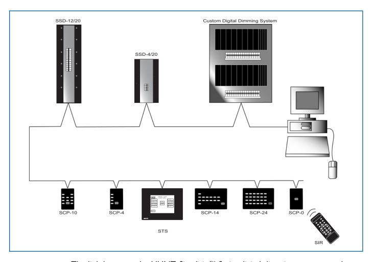
The link between the HUNT Simplicity<sup>™</sup> Series digital dimming system panels and control devices is key to the system configuration. This physical link is a cable called the data highway where this cable carries all information between the dimming panels and control devices.
