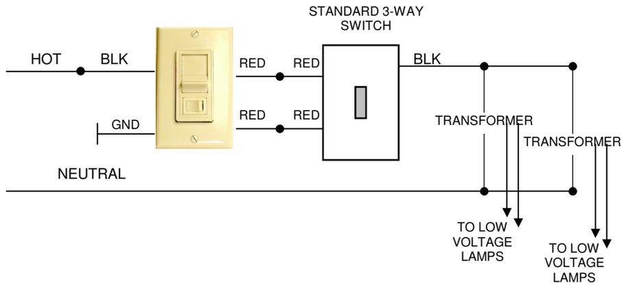
**Typical Compatible Magnetic Low Voltage Transformers**
