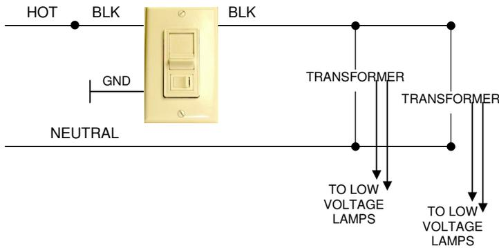
**Typical Compatible Magnetic Low Voltage Transformers**
