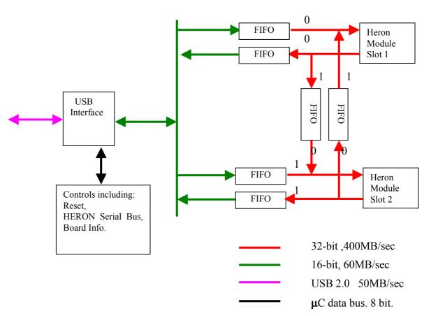
HERON modules are designed to be interfaced to carrier boards that provide synchronous FIFOs.
