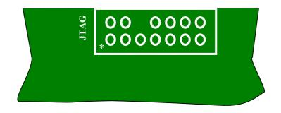
This connector is the standard pinning for a 14 way JTAG header so it accepts the cable supplied with, for example, a TI XDS510 or 560. The HERON-BASE2-FIFO is only ever a JTAG slave.
