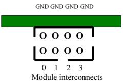
Fitting HERON modules to your carrier is very simple. Ensure that the module carrier does NOT have power applied when fitting modules, and normal anti-static precautions should be followed at all times.
