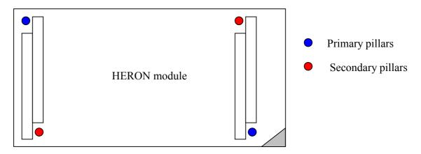
The Carrier card will probably only have spacing pillars fitted to the primary location for each HERON slot. The pillars for the secondary locations will be supplied as an accessory. The reason for this is that the legacy GDIO modules cannot be fitted if the secondary pillars are in place.
