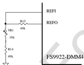
Diagram 11: The Utility of Internal Base Power Source
