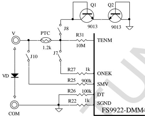
Diagram 28: Diode Test
