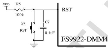
Diagram 13: Reset Circuit
