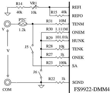
Diagram 22: Voltage Measurement
