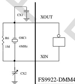
Diagram 14: Oscillation Circuit
