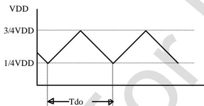
Diagram 31: Capacitance Measurement
