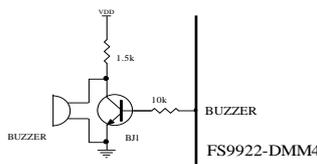
Diagram 16: High Resistance Buzzer Connection
