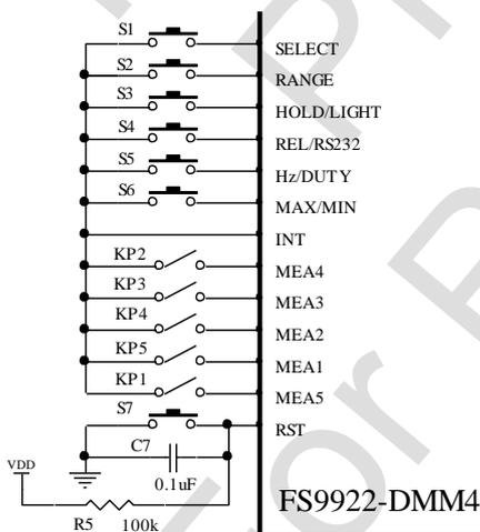
Diagram 17: Mode Switch and Function Control Circuit
