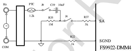
Diagram 34: RPM Measurement
