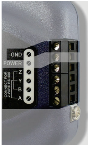
Figure 3: Terminal Block RS-485 Connections
