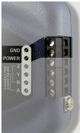
Figure 1: Terminal Block Power Supply Connections
