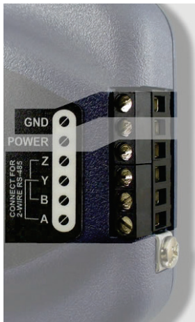
Figure 3: Terminal Block RS-485 Connections
