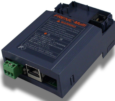
Figure 1: OPC-E1-ETH Interface Board
