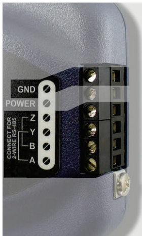
Figure 3: “RS-485 B” Terminal Block Network Connections
