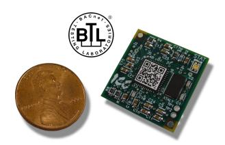
Miniature serial communication module for OEM platforms
