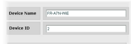
Figure 27: BACnet Device Identifiers
