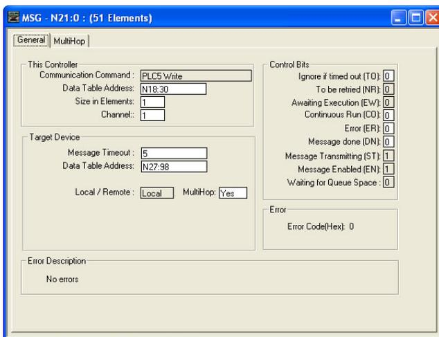
Figure 124: MSG Configuration for Writing
