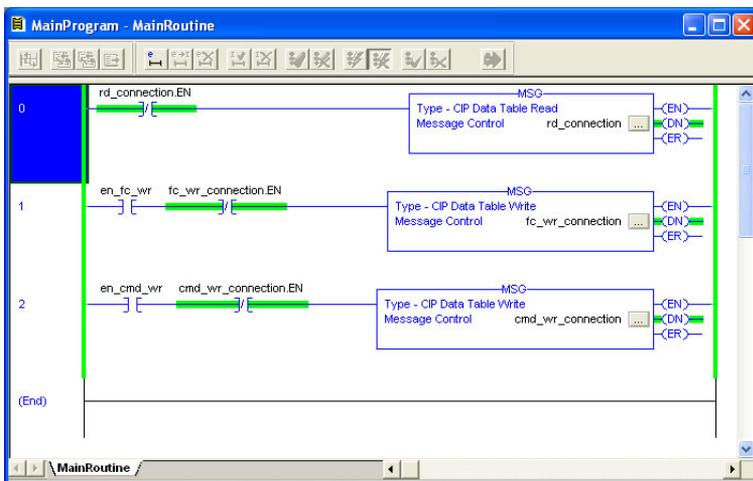
Figure 110: Reading and Writing via MSG Instructions
