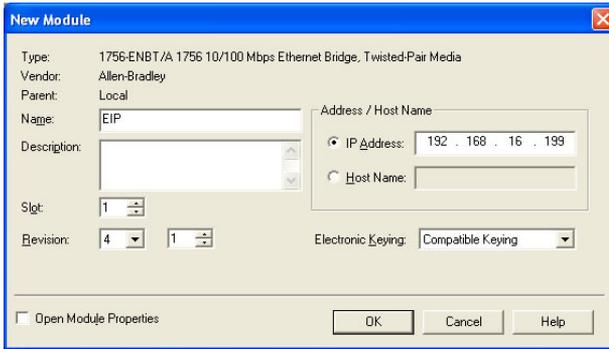
**Figure 79: Configuring the New Module**
