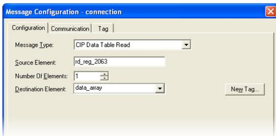
Figure 108: Read the Inverter's Operation Status Register
