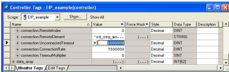
Figure 97: Reduce the UnconnectedTimeout Value
