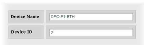
Figure 24: BACnet Device Identifiers
