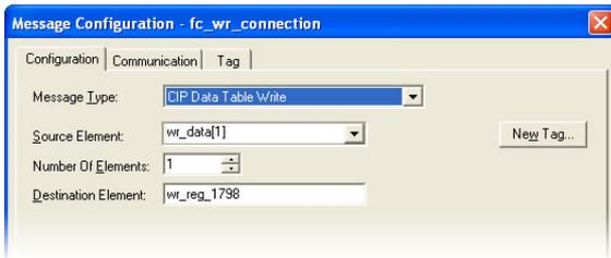
Figure 111: MSG Configuration for Writing
