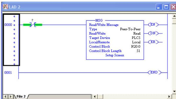
Figure 118: PLC Program after MSG Instruction Configuration
