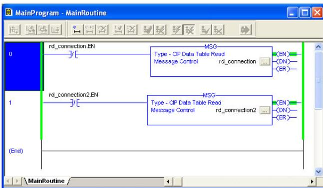
Figure 109: Reading Via Multiple MSG Instructions
