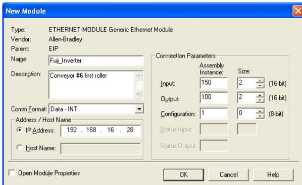
**Figure 82: Interface Card Module Properties**
