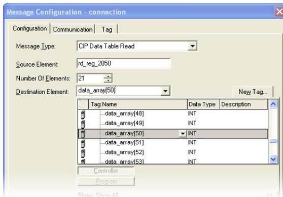
**Figure 102: Selecting the Destination Element**
