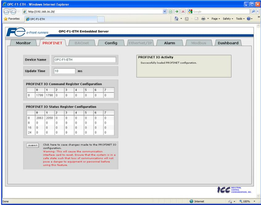
Figure 17: PROFINET Tab
