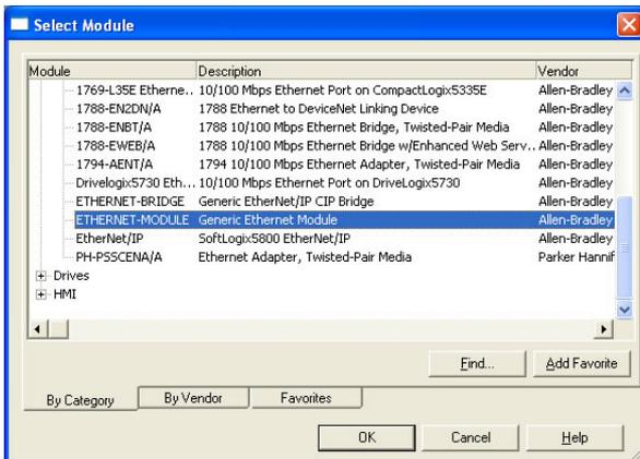
**Figure 81: Adding a New Generic Ethernet Module**
