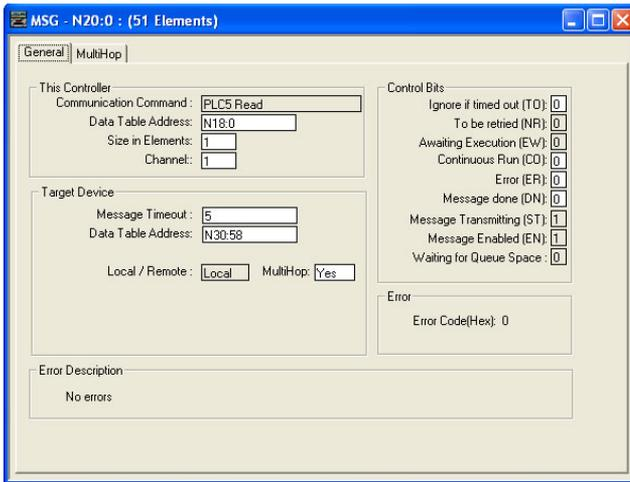
Figure 121: Read the Inverter's Output Frequency Register
