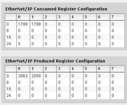
Figure 37: EtherNet/IP Class 1 (I/O) Data Configuration
