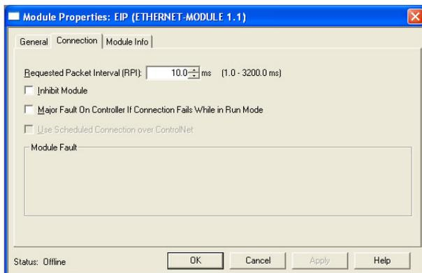
**Figure 83: Interface Card Module Properties Connection Tab**
