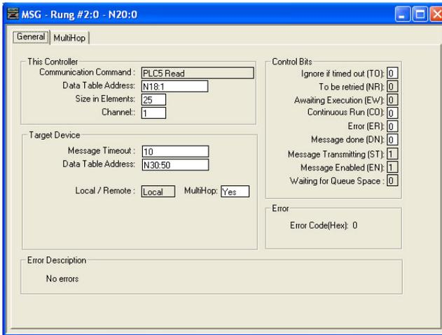
Figure 116: MSG Configuration, "General" Tab
