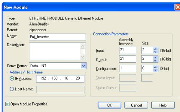
**Figure 91: AC/DC Drive Profile Generic Ethernet Module Configuration**
