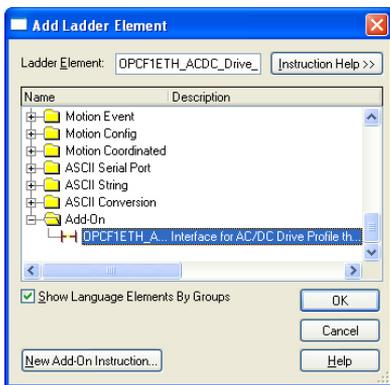
**Figure 94: Add AC/DC Drive Profile AOI**
