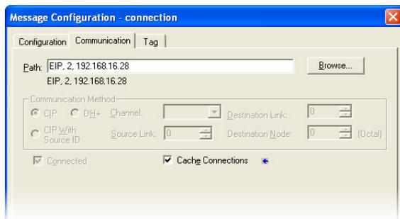
**Figure 103: Setting the Communication Path**
