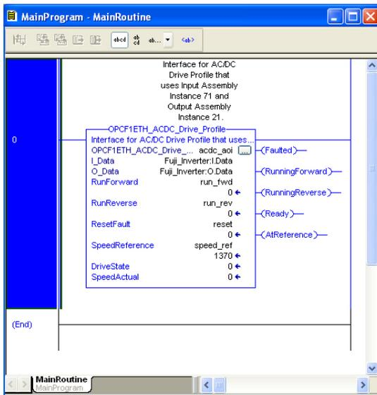
Figure 95: Configure AC/DC Drive Profile AOI
