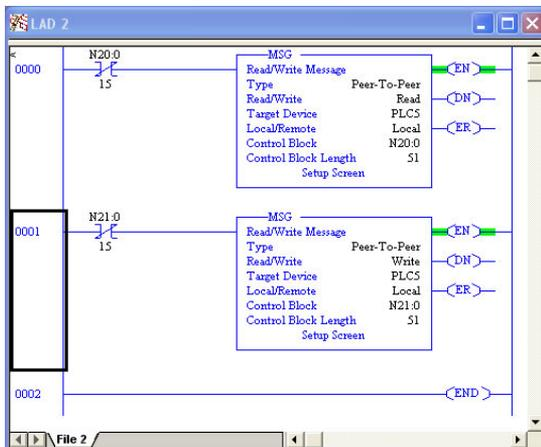
Figure 123: Reading and Writing via MSG Instructions
