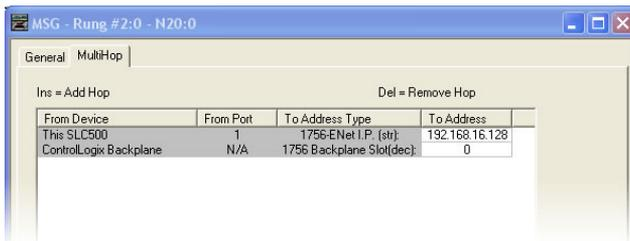
Figure 117: MSG Configuration, "MultiHop" Tab
