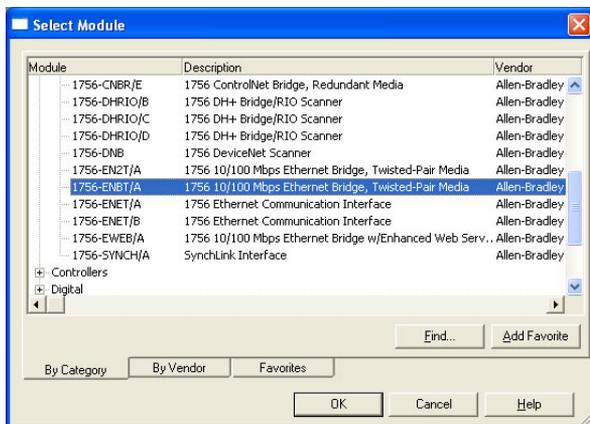
**Figure 78: Adding a New 1756-ENBT/A Module**
