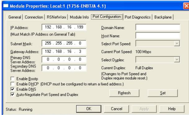
**Figure 80: Confirming the Module's Properties**
