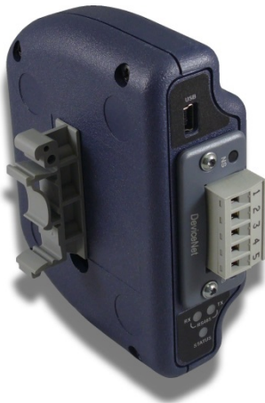
Figure 8: Unit with Attached DIN Rail Adapter
