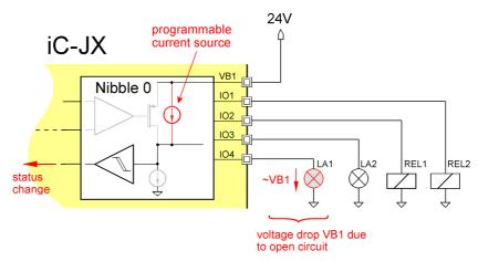
Figure 2: System diagnosis using programmed current sources
