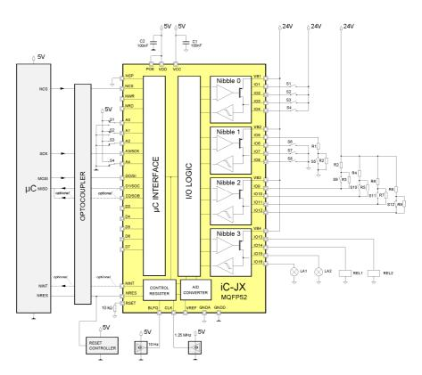
Figure 1: iC-JX in a typical application environment
