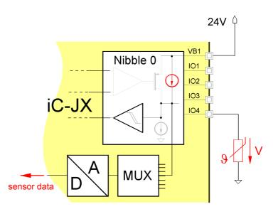
Figure 3: The use of the A/D converter for sensor evaluation
