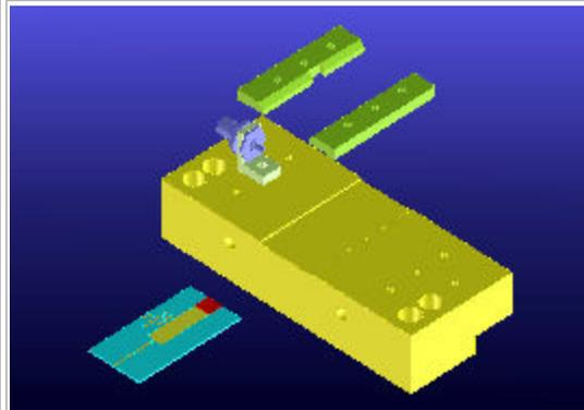
50 to 11 Ohm launch on 25 mil Alumina exploded
