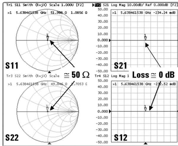
Figure 6. S-parameter measurement result of the Line
