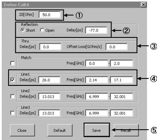
**Figure 3. Standard coefficient input screen**
