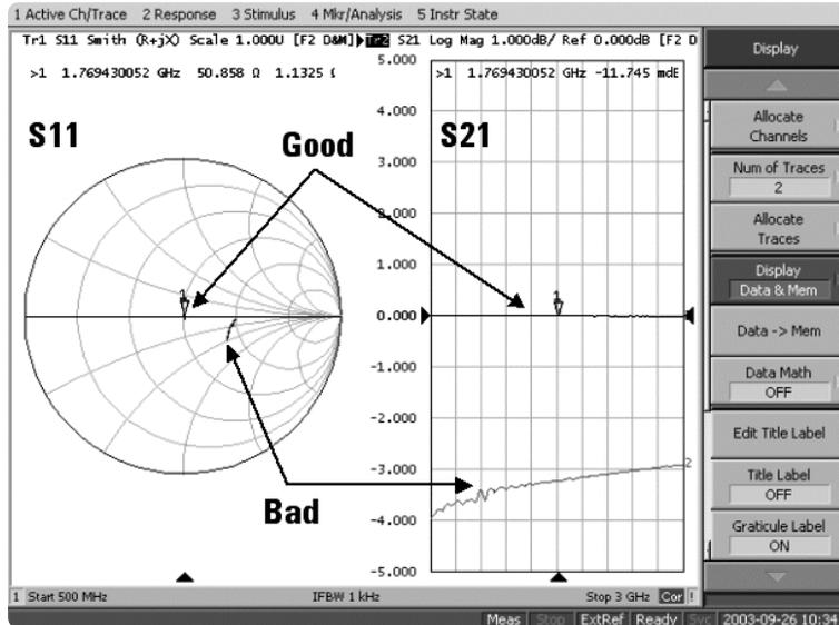
Figure 10. Confirmation of device contact condition
