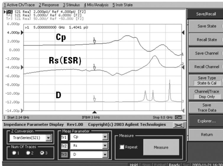
Figure 12. Measurement results of SMD capacitor using impedance parameter display software
