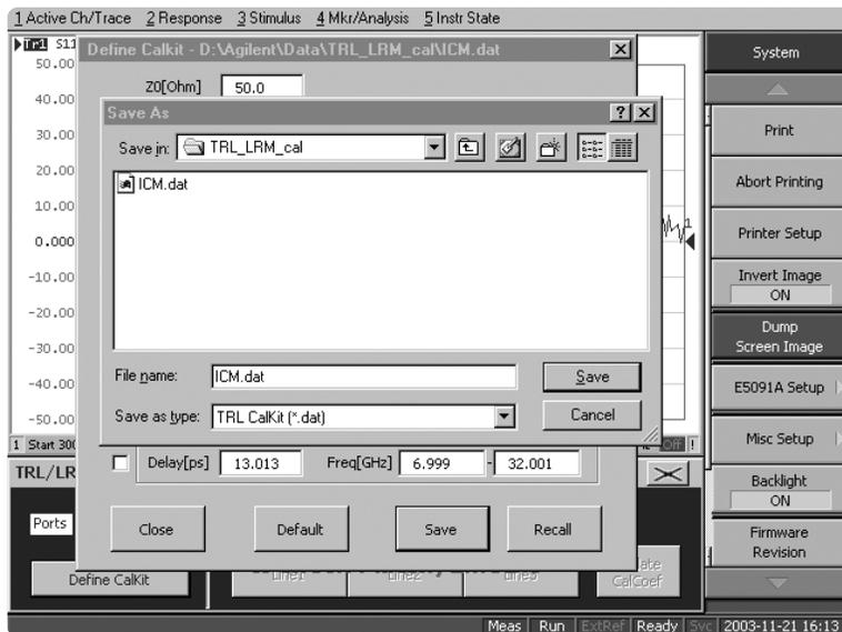
**Figure 4. Save the standard coefficient of TRL calibration**
