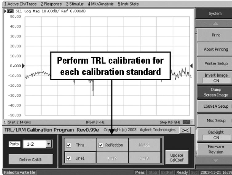
Figure 5. Performing TRL calibration
