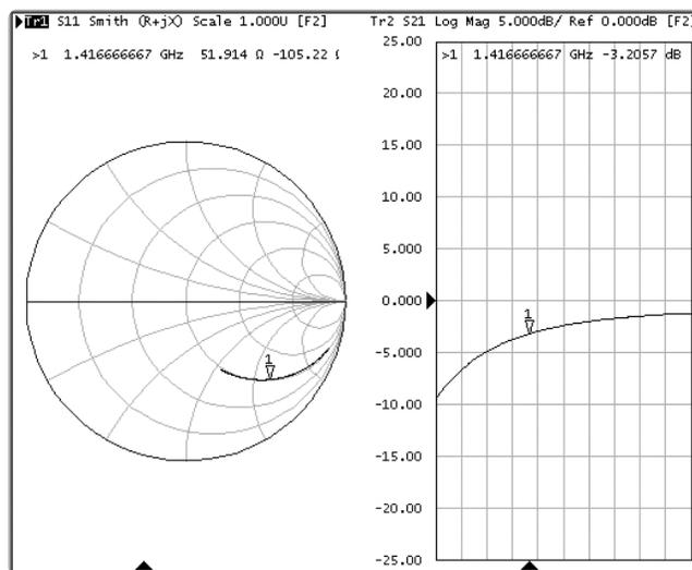
Figure 11. SMD capacitor measurement (1pF, size 1005 mm/0402 inch)
