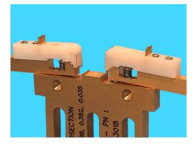
The adjacent picture shows the DC Probes in the open position. Insert the MMIC Carrier Assembly, and simply push the Lever Assembly forward. It will close automatically.
