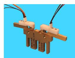
The MMIC Midsection Adapter holds the MMIC Carrier Assembly and provides the DC inputs (10 lines) to power and control the DUT. Two cable assemblies connect the unit to the power supplies.
