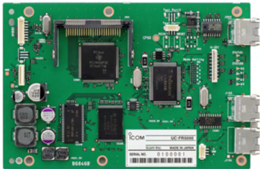
UC-FR5000 IDAS™ Trunking/Network Controller
