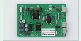
UC-FR5000 (#12) dPMR Mode 2 Network Controller For dPMR Mode 2 IP networking (Cannot be installed in Mode 3 version)
