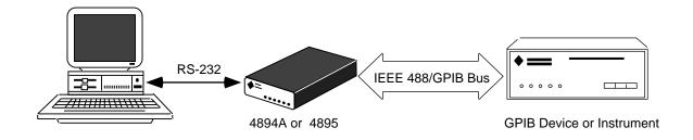
Figure 1 Serially controlling a GPIB Device
