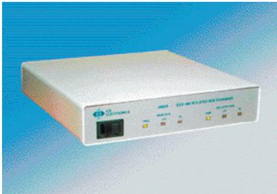
Bus Isolator, the Model 4860A, that provides increased bus isolation and noise protection while expanding the number of devices beyond the specification limit of 14 devices. The Model 4860A isolates instruments from the bus controller, eliminates ground loops and noise, and lets instruments 'float' up to the potential of their test signals.
