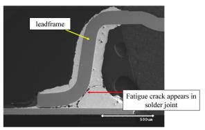
crack due to this CTE mismatch that occurred in a test chamber after extensive temperature cycling between -40°C and 125°C. This could result in an intermittent connection at the solder joint.
