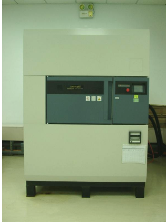
Figure 3-9 HITACHI Cycling Oven, for TCT test
