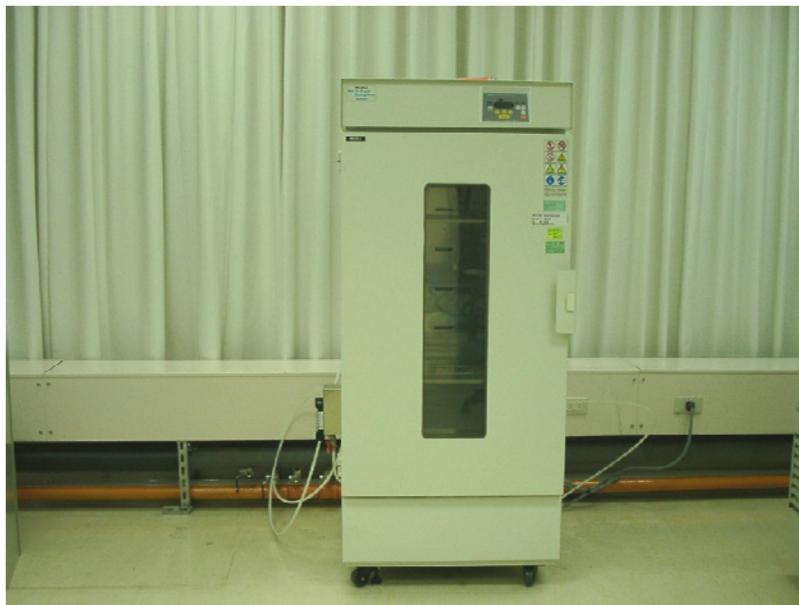
Figure 3-10 ISUZU High Temp Oven, for HTS test
