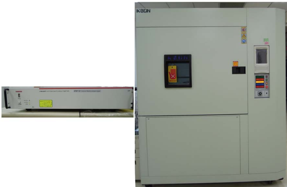
Figure 3-12 KSON Temperature cycle chamber and Keithley system switch/multimeter, for solder joint life test
