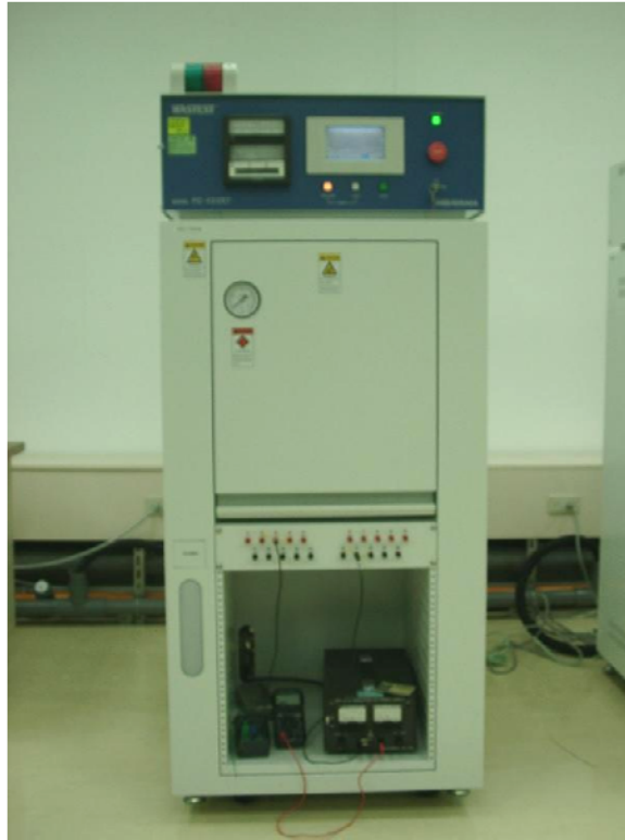
Figure 3-7 HIRAYAMA Pressure Oven, for HAST test
