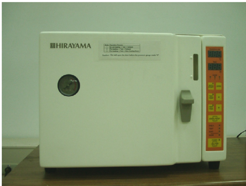
Figure 3-8 HIRAYAMA Pressure Oven, for PCT test
