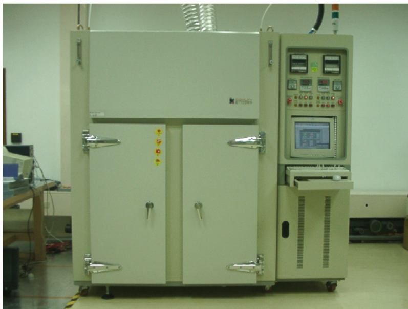
Figure 3-6 Signality Burn-in Oven, for HTOL test
