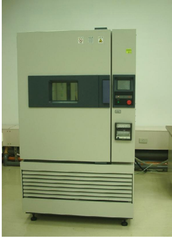
Figure 3-11 HITACHI Humidity Oven, for THS test
