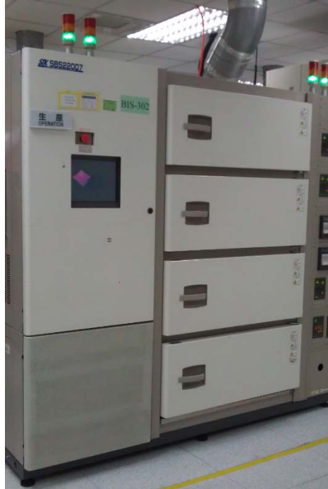
Figure 3-5 STK Burn-in Oven, for HTOL test
