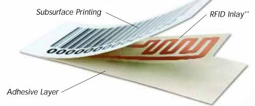
Why are these tags so durable? Every one of our RFID tags utilizes a construction that encapsulates the RFID inlay within the layers of the label – protecting it from environmental conditions that could affect its performance. Each product also features digital subsurface printing that showcases company information and/or logo and may include variable data such as bar code and/or human readable numbers allowing users to utilize both bar code and RFID technologies.
