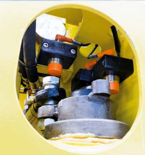
Safe lifting: Inductive ifm sensors monitor if the container is safely locked in the spreader.
