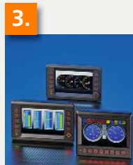
3. Dialogue module PDM360 NG 7.0" TFT graphic display for operation, visualisation and parameter setting of the functions of the vehicle.
