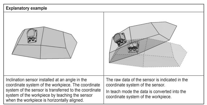
The example shows a rotation of 30° about the y axis of the coordinate system of the workpiece.
