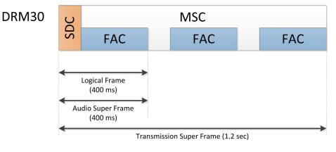
Multiplex structure of DRM30 and DRM+ transmission schemes. Note the different timescales for DRM30 and DRM+.
