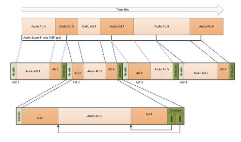
Packing of Audio AUs into the DRM Audio Super Frame (ASF) Transport
