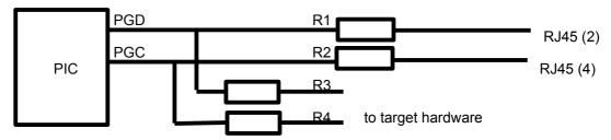
Select the value of R3 and R4 in the range of 2k ... 10k and R1, R2 in the range of 470 to 1k, then it will work, if the following hardware could sink and source the current from programmer. If programmer is in idle state (non programming state) the pins RJ45 (2) and RJ45 (4) are in tri state which is high impedance. This means that signal coming out of the targets hardware will not effect.
