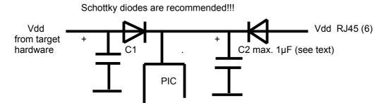
Capacitor C2, which is connected close to the PIC, may <u>not exceed 1µF</u>, because the slope becomes to flat. To enter program/verify mode the slope may not slower than 1 µsec. If EMC makes C2 greater than you must split it in to capacitors which is also recommended by EMC (e.g.  $C1 = 10\mu$ F and C2 = 100nF). This results in two resonants peaks.
