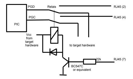
A less comfortable but also save solution is replaceing the relais by a simple switch or jumpers.
